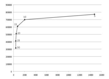
**Fig. 6.** Impact of the minimum overlap parameter on correctness of the read merging algorithm. The horizontal axis shows the number of incorrectly merged read pairs, and the vertical axis shows the number of correctly merged read pairs. The minimum overlap value (in base pair) is shown on the graph.
